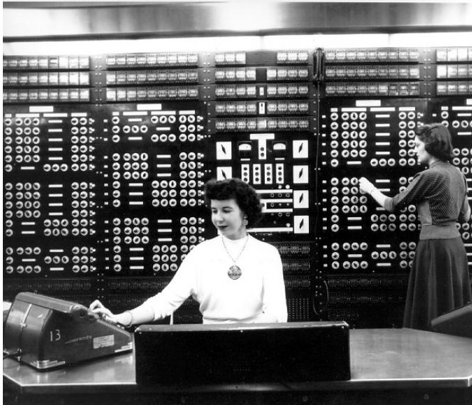
Figure 8-6. Harvard Mark II relay computer (1947) Courtesy of IEEE Annals of History of Computing
