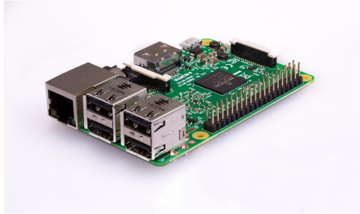
Figure 1-1. Raspberry Pi 3 Model B single-board computer fits on a board 3.5 by 2.25 inches
